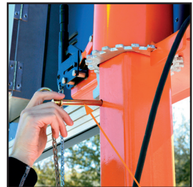
Remove the Locking Pin before lowering.
